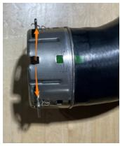
**13.** Disconnect the smaller upper coolant reservoir hose from the radiator.
