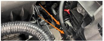
**22.** Remove the 4x 10mm (2x per side) fan shroud bolts securing the fan shroud to the radiator and lift it out of the vehicle.
