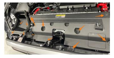
5. Remove the 3x 10mm bumper bolts at the top of the bumper. Then, disconnect the 2x electrical connectors on the passenger side of the bumper. Vehicles with a front bumper camera will also have another electrical connector on the driver's side of the bumper which also must be disconnected.
