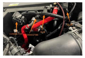
**16.** Disconnect the small upper radiator hose from the radiator and the second coolant hose connected to the transmission cooler. (See image on the right)
