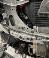
**30.** Reinstall the 2X side ducts on the core support and install the 3x (6x total) push clips on each side.
