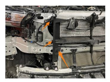
**12.** Remove both charge pipes from the vehicle, disconnect the quick disconnect ends by pushing the wire clip apart as shown, and pull away from the connection on the intercooler, turbo outlet, and throttle body.
