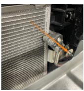
24. Remove the 6x 12mm bolts holding the radiator to the core support. Remove the 4x lower bolts first and then the 2x upper bolts. The radiator should be held up by hooks above the top bolts. Then, remove the radiator and intercooler assembly from the vehicle. Make sure that the radiator does not get stuck on the A/C line on the driver's side.
