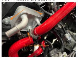
**18.** Clamp off the two transmission lines connected to the radiator and then remove the lines from the radiator. Be careful to clean up any transmission fluid that comes out. It is helpful to cap off the fittings on the radiator to prevent leakage during removal.
