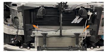
31. Take the Mishimoto rubber duct and line it up with the 2x holes in the side ducts and the hole in the black middle bracket, then place the included flat bracket underneath the duct and thread in the included 4x 8mm bolts into the threaded holes on the bottom of the intercooler. Tighten each bolt hand tight and then tighten each bolt to approx. 50 in-lbs. Check to make sure that none of the bolts have become loose during this process as the rubber depresses causing the bolt to come loose.
