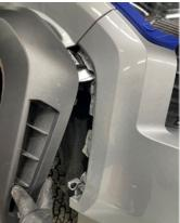
8. Remove the 6X 10mm bolts securing the bottom of the bumper, then move the felt wheel well liners out of the way and remove the final 2X 10mm bolts that secure the bumper to the vehicle.
