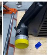
26. Make sure that the bushings are pre-installed onto the passenger side of the Mishimoto intercooler. If they are not, first install the rubber part of the bushing and then install the metal insert from the front ("M" logo side). Install the Mishimoto intercooler onto the radiator. There should be hooks on the top mounting points to hold the intercooler in place while
